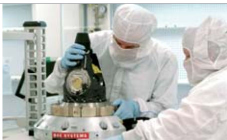
Terminal High Altitude Area Defence (THAAD) BAE Systems is responsible for the development of the infrared seeker head on the THAAD missile system. The THAAD missile system is designed to defend against attacks from short and medium-range ballistic missiles. Here assemblers at BAE Systems in Nashua, New Hampshire, install a THAAD seeker forward ring assembly into a vibration test fixture.
